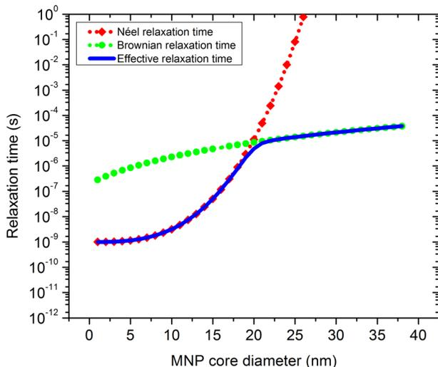
FIG. 2. Néel, Brownian, and total effective relaxation time as function of MNP core diameter,  $T = 293$  K. Viscosity of the MNP solution is 1 cp.
