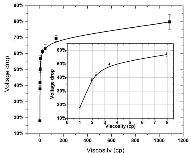
FIG. 5. Voltage drop in percentage vs. viscosity for MNPs in nine mixtures at 20 °C.
