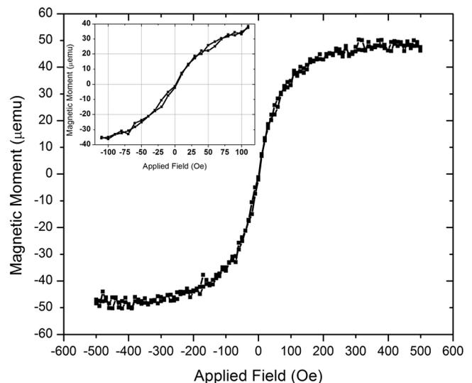
FIG. 1. Magnetization curve of iron oxide nanoparticle suspensions (SHP-25 from Ocean NanoTech) at 20 °C measured by a Vibrating Sample Magnetometer (VSM).
