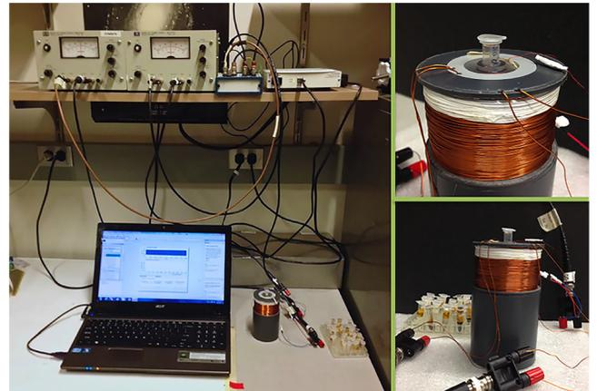
FIG. 3. Detection-coil based MNPs detection system experimental setup.
