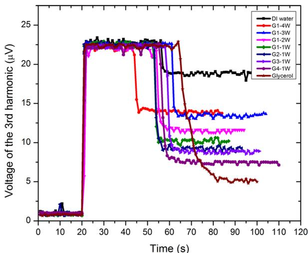
FIG. 4. The real-time voltage signal of the 3rd harmonic for MNPs in nine mixtures at 20 °C.
